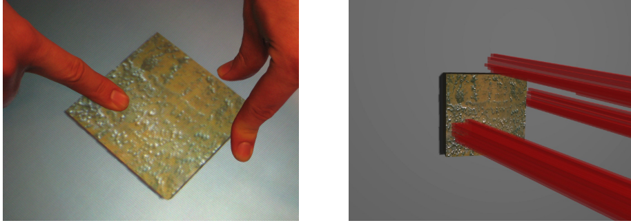
Figure 2.5: The physics-based interaction technique by Wilson et al. [Wil08]. The contours of the contacts are extended into the virtual world as bundles of stick-shaped particles.
