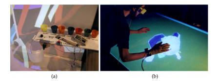
Figure 2: The table interface used in the 3D CavePainting system [Keefe et al., 2001] (a) and a user interacting with the Responsive Workbench [Cutler et al., 1997] in the Surface Drawing [Schkolne et al., 2001] system (b).
