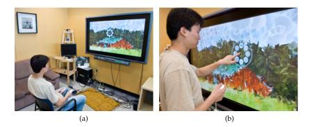
Figure 11: Bimanual interaction techniques permit a seamless transition from remote pointing (a) to direct-touch (a).
