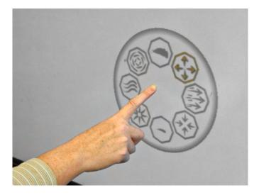
Figure 18: When touching the screen the tools menu appears at the touch location. The repel tool is selected with the Nunchuk.
