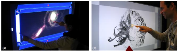
Fig. 1. Two case studies for a 3D visualization exploration widget that allows users to control the view in 7 degrees of freedom (DOF): (a) touch interaction with an astronomical simulation; (b) exploration of an illustrative 3D medical visualization.
