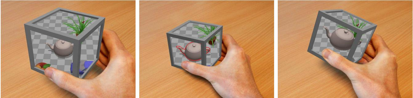
Figure 1: Our concept of a *tangible volume* consists of a fully portable and self-contained device, entirely covered with screens. A virtual scene can be seen “through” the volume of the device (left image). This volume can be directly positioned within the virtual scene (middle image), and used to grasp and manipulate virtual objects (right image). A cubic-shaped device is shown here for illustration, but other volume shapes can be used.
