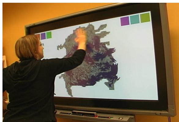
**Figure 6:** Glyph de-emphasis & erasing using the flat hand.
