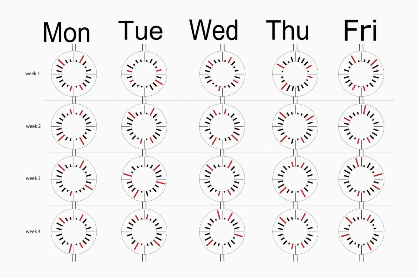
One is a radial bar chart showing noise levels for each working day of the month. The circular graph is divided into four me slots between 9 am to 9 pm. In each me slot the noise level is drawn as an average for thirty minutes and times that exceed a critical threshold are marked in red.
